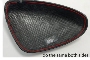
3.After that add adhesive at the lines as is shown in the photo (We recommended Black Bodywork Silicon Glue as adhesive such as 3M or Wurth).
