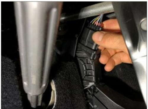
• Connect the connector with the female pins of the Marelli harness to the potentiometer (Fig. 2)
